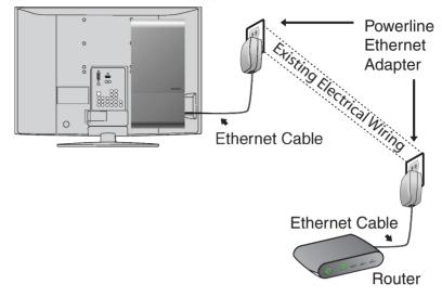
**Option 2. Powerline Ethernet Adapter Connection**
